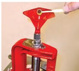
**CAUTION** After charging the case, the only operation that should be done is to seat the bullet. Never try to seat a primer after powder has been added.
