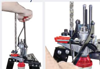
Size cast bullets as fast as you can pull the lever with the BREECH LOCK BULLET SIZING KIT # 91532 and diameter specific bullet sizer and punch.
