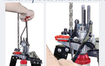
Size cast bullets as fast as you can pull the lever with the BREECH LOCK BULLET SIZING KIT # 91532 and diameter specific bullet sizer and punch.
