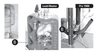
Raise carrier to the mid stroke position, snap bead chain into the disconnector slot.
