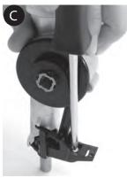
**C:** Re-install 6-32 Phillips screw to secure disconnector.
