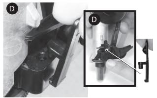
**D**: Clip on latch lever to slider drop tube. Install the pin in the screw hole
