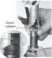
Insert case into shell holder and raise ram. Thread powder measure and charging die into the press until you feel it stop turning, turn the powder measure in further until the slider drop tube raises to the dispense position. Finger tighten lock ring. If the powder measure is not in a convenient position, loosen the swivel adapter and rotate.
